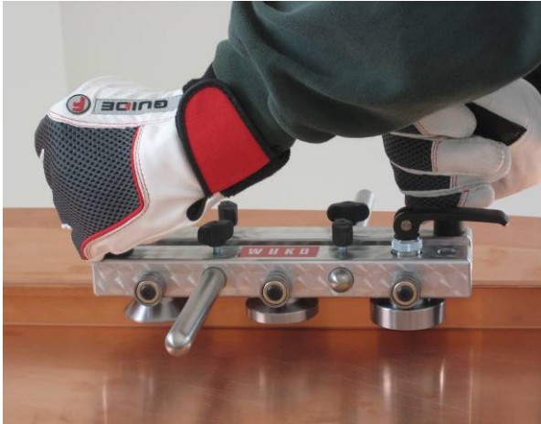
Move the tool forward by using handholds
